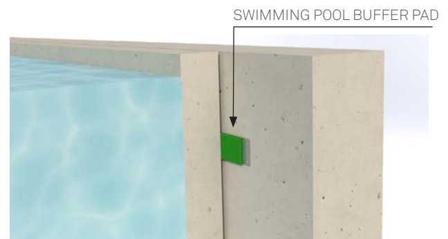
SWIMMING POOL BUFFER PAD INSTALLATION EXAMPLE
